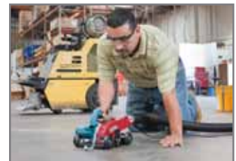
Free-hand scoring using roller guides
